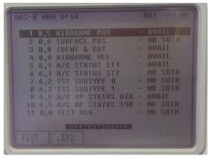
AIRBORNE POS. Confirm the ICAO code (AA), Position (LAT/LON), Altitude and NIC/Rc are correct.
