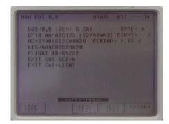
3. A/C STATUS ST1. Confirm the ICAO code (AA) and Mode A code are correct. Enter code 7500, 7600 or 7700 on the T2000ADSB and ensure the EMERG/PRIOR Code is correct.
