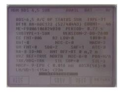
Simulate the aircraft being in the air (follow the aircraft maintenance manual or often the easiest way is to enter Program Mode on the T2000ADSB and change the AIR/GND Logic from Norm to Rev or vice
