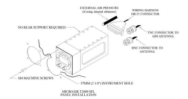
The T2000ADSB weighs only 600g (1 lbs). The four M4 x 12mm machine screws are sufficient to support the transponder. No rear support is required unless the panel structure itself is too weak to support the load.
