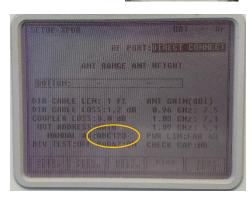
Ensure ADSB Version 2 is selected in the T2000ADSBs Program menu (this is required because the IFR6000 does not yet support Version 3 messages).
