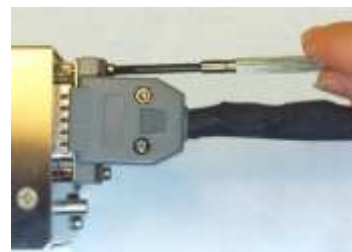
Locking bolts tightened
