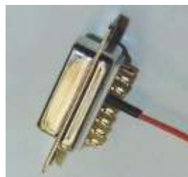
Soldered with heatshrink
