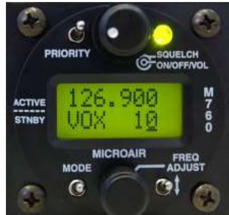
Press the mode switch until the VOX adjust screen is displayed, and set the VOX threshold to the desired level. It may be necessary to readjust this level when the aircraft is operating at full power.
