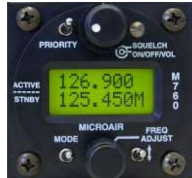
*While receiving a signal on the active frequency - the standby channel is **NOT** monitored.*
