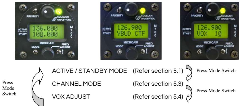
If the internal VOX intercom has been disabled in the program mode menu the intercom adjust mode will be skipped. See section 6.2 to enable / disable the internal VOX intercom.
