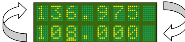
If the remote memory button is held down for 3 seconds while in the active / standby mode, the monitor function is activated. Refer to section 5.2 for complete details on monitor function.
