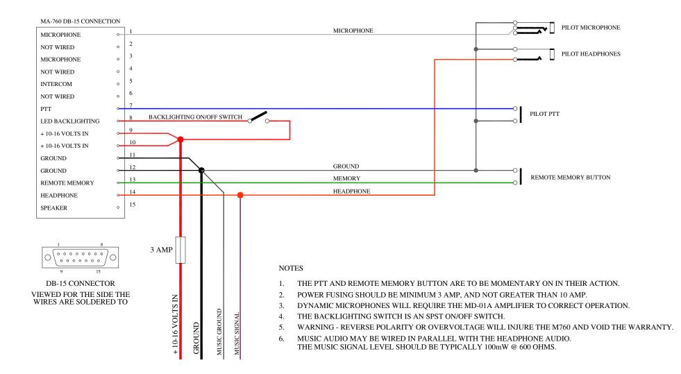
MICROAIR M760 (REV N) TRANSCEIVER WIRING DIAGRAM SINGLE SEAT TRIKE INSTALLATION
