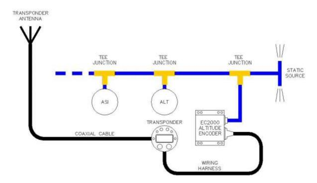
After installing, remove the dust plug from the NPT fitting, and connect the static hose line ensuring the NPT connector is sealed using thread tape or an appropriate sealer (not silicone). Connect the wiring harness terminated with a DB-15 from the transponder, to the DB-15 fitting adjacent to the NPT fitting on the EC2002. Ensure that the DB-15 thumbscrews are secured to the hex-nuts on the EC2002's case.
