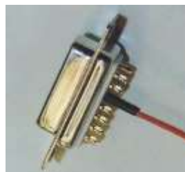
Soldered with heatshrink
