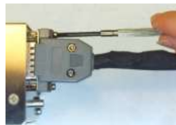
Locking bolts tightened
