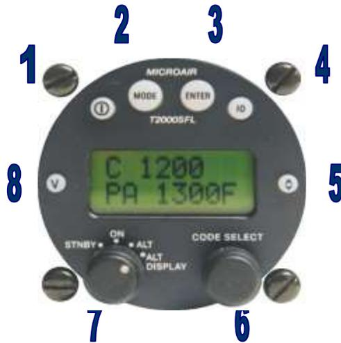
All of the keys are covered in a soft rubberized plastic, which is backlit with the display. When the key is pressed a small click can be discerned. The selected function will operate on the release of the key.
