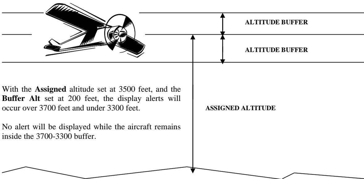
If the aircraft climbs or descends outside the altitude buffer limits, a **Hi / Lo** warning is displayed on the lower line.
