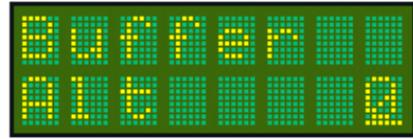
If the **ALTITUDE** option in the **PROGRAM MODE** is set to **FEET** the **Buffer Alt** increments are in feet. If **ALTITUDE** is set to **METRES**, the **Buffer Alt** increments are in meters.
