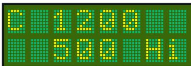
**T2000SFL** advises the pilot that the aircraft is 500 feet above the **Assigned** altitude. If the **Alert Tone** function is set on, an audio warning tone is heard.
