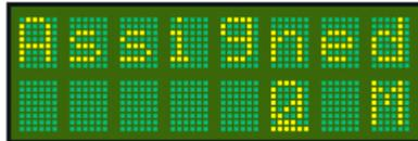
When the **Altitude** option of the mode menu is set to Meters, the **Assigned** altitude is adjusted in Meters.
