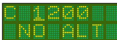
The **T2000SFL** will transmit the encoder altitude (pressure altitude) only, in accordance with normal mode C operation. The adjusted **QNH / Baro** altitude is *never* transmitted.
