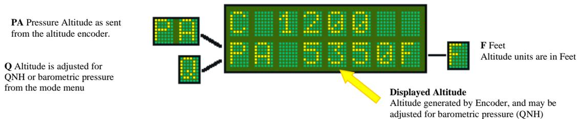
The altitude value is rounded to the nearest 10 foot increment. Be aware that where the altitude data input is received in increments of 100ft the rounding can only be in 100ft steps also.
