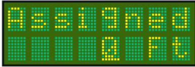
When the **Altitude** option of the mode menu is set to Feet, the **Assigned** altitude is adjusted in feet.
