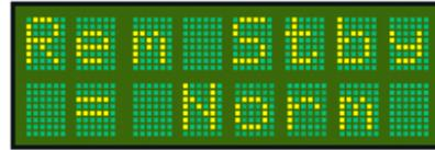
If the remote switch releases the T2000SFL from standby by closing, the operation is **NORM** (normal).
