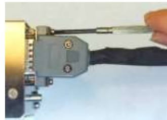
Locking bolts tightened
