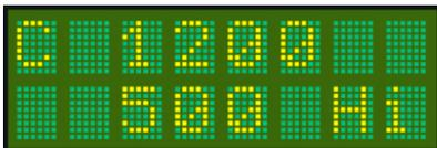
**T2000SFL** advises the pilot that the aircraft is 500 feet above the **Assigned** altitude. If the **Alert Tone** function is set on, an audio warning tone is heard.
