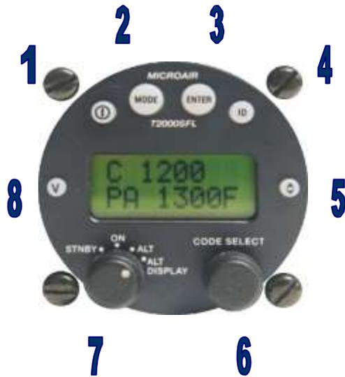
All of the keys are covered in a soft rubberized plastic, which is backlit with the display. When the key is pressed a small click can be discerned. The selected function will operate on the release of the key.
