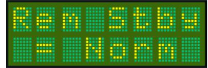
If the remote switch releases the **T2000SFL** from standby by closing, the operation is **NORM** (normal).
