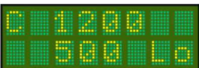
**T2000SFL** advises the pilot that the aircraft is 500 feet below the **Assigned** altitude. If the **Alert Tone** function is set on, an audio warning tone is heard.
