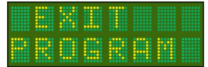
The user can exit the **PROGRAM MODE** menu at any time, from any menu item, by pressing the **toggle** key.
