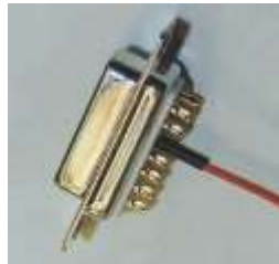
Soldered with heatshrink
