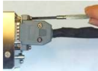
Locking bolts tightened
