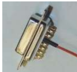
Soldered with heatshrink
