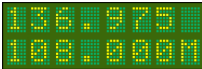
Monitor Mode Monitoring on STANDBY frequency
