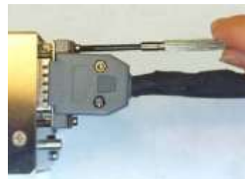
Locking bolts tightened
