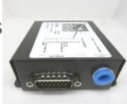
The EC2002 accurately reports the aircraft's altitude over a calibrated altitude range of -1000 to +35,000ft. The altitude output can be via the 10 line Gillham "Gray" code, or a 2 line serial data output.
