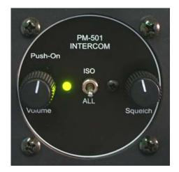
The PM-501 features an entertainment (music) input, which is typically wired out to a jack on the panel. This allows the pilot or passengers to input music into the intercom system. The music will "mute" to a low volume level when there is intercom activity.
